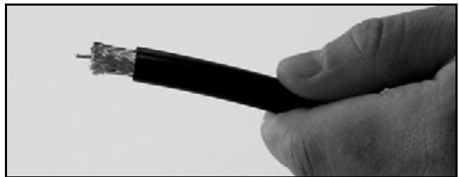
Figure 57: Cable Stripped, Exposing Dielectric
