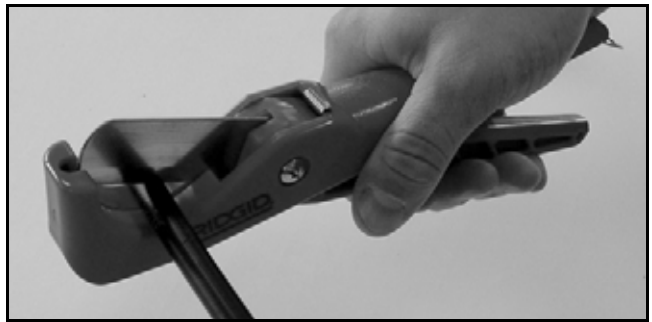
Figure 51: Cutting the Cable
