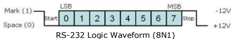
The baud rate is the communication speed that measures the number of bit transfers per second. For example, 19200 baud is 19200 bits per second.
