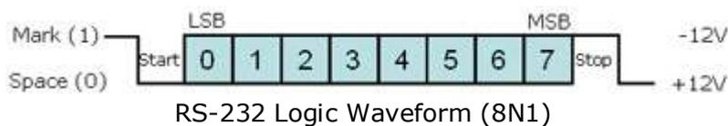
The graphic above illustrates a typical RS-232 logic waveform (Data format: 1 Start bit, 8 Data bits, No Parity, 1 Stop bit). The data transmission starts with a Start bit, followed by the data bits (LSB sent first and MSB sent last), and ends with a "Stop" bit.
