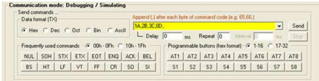
Use the above example to control a projector (turn ON the projector), key in the complete command string "1A,2B,3C,0D," into the Send\_Command\_Pane as shown above (note: You need to add a "," sign after each command code), and then click on the "Send" button...
