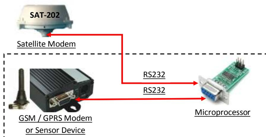
The GSM / GPRS modem is a highly flexible plug and play modem for direct and easy RS232 integration. The Microprocessor can either be a stand alone product or part of the integrated GSM / GPRS or other Sensor solution.
