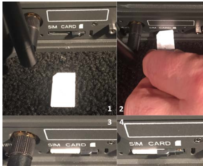
Figure 3-4 Installing SIM Card and Engaging the Lock
