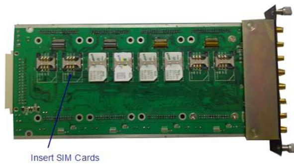
Figure 2-2-1 Push in the GSM user board
